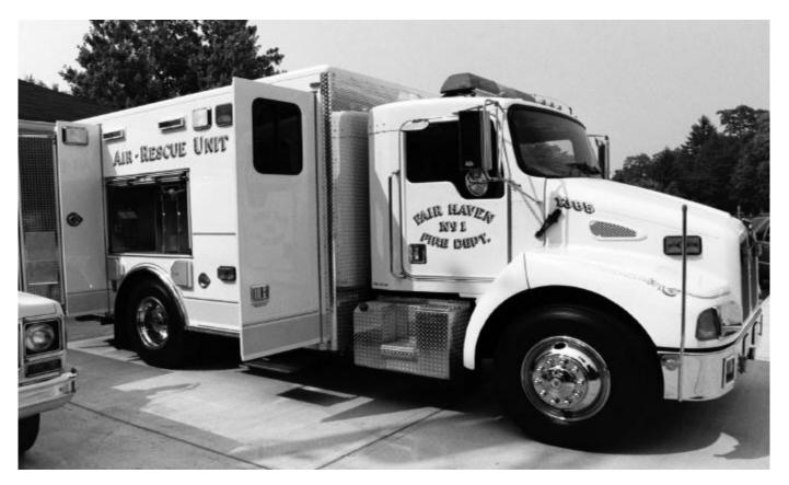
The Fire Company's New Air-Rescue Unit includes a lighting tower that provides 10-kilowatts of area lighting, has an enclosed cab for firefighters as well as the driver, and includes numerous compartments for rescue tools and other essential equipment.
